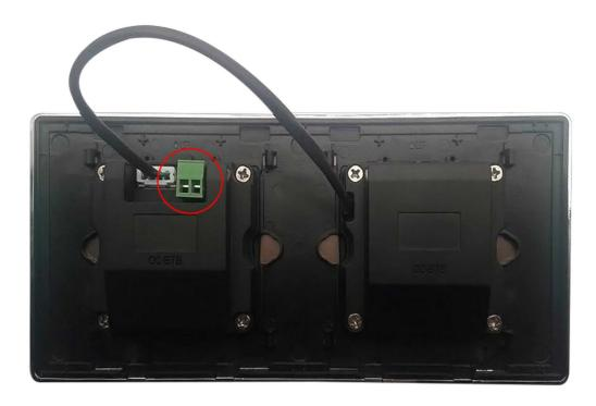
4. Mount the faceplate wall-mount phone by clipping onto the clip-in plate after fasten the telephone wire to the back connector.
